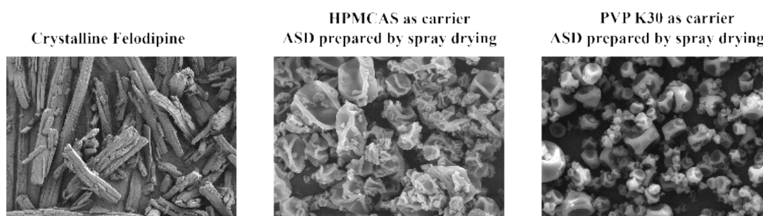
Figure 4: SEM Comparison of Crystalline Felodipine and Felodipine ASDs Prepared with Different Carriers via Spray Drying
